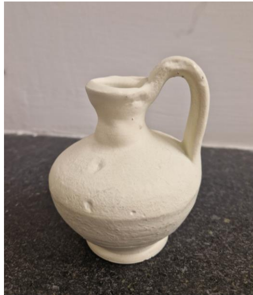
Figure 4: vase made with SLA 3D printer.
